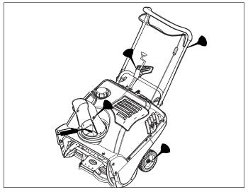
Figure 10. Lubrication points
